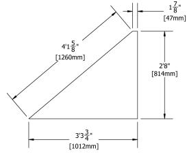
\*All Dimensions in Feet & Inches and [mm] Made to Fit 2"Ø Chords/Tubes
