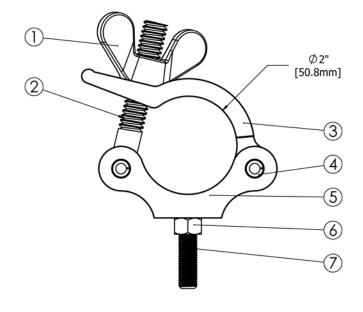
Total width when closed (including wing nut): 4.8" [122mm]
