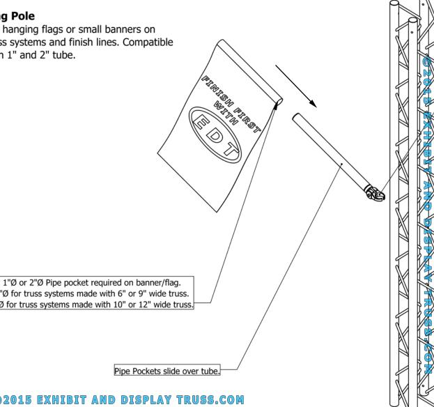
Flag pole tube available with 1" or 2" Extender Hook Clamps for 1"Ø or 2"Ø Chords. Extender Hooks swivel and allow flag to be on angle and moved to desired height along truss.
